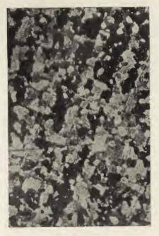
Fig. 1. (x 80 Diameters. Vertical Illumination.) Cast Tin Filed and Etched. Showing change in structure.
